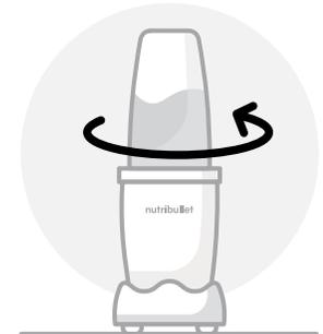
Unlock the assembly by gently pushing and untwisting the cup counterclockwise.
